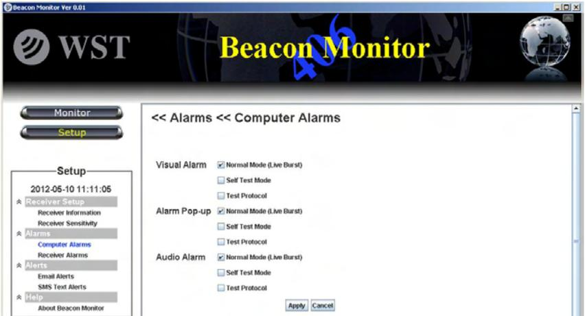
There are three alarm notification methods on the computer; Visual Alarm, Alarm Pop-up, and Audio Alarm. When an alarm notification is triggered by a received burst, an Alarm Reset button appears below the Setup button. To clear the alarm, click on the **Alarm Reset** button.
