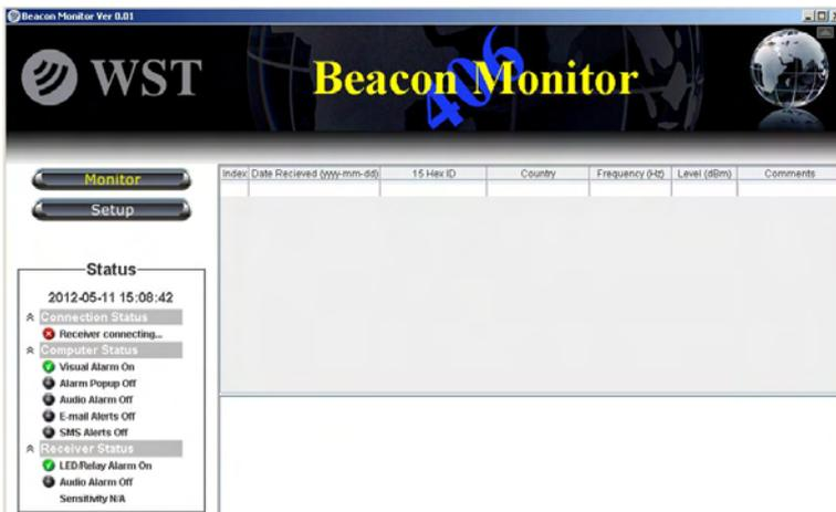
The Connection Status in the Status section shows a red X, indicating the receiver is not connected.
