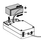
**3** Pull out the battery and disconnect the battery wires.
