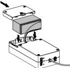
3 Insert the battery back into the compartment.
