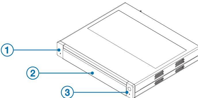
1. Switch-on button with switching-on LED marker;
