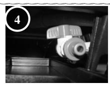
The discharge valve is closed when the valve handle is horizontal.
