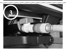
Screw the orange disconnect adapter to the male hose. Slide the orange quick connect onto the discharge valve. Make sure that the connection is secure.
