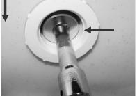
Clean this area, using low foaming soap and disinfectant, with a brush. Remove all visible residue and rinse with clean water.
