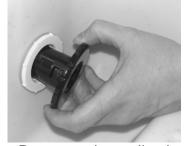
**Step 2:** Remove the adjusting cover. This should pull out.
