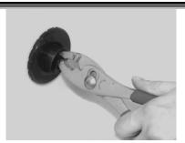
**Step 1:** Remove the jet eyeball using the pliers. Pull forward with a quick tug.
