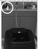
Route the discharge hose into a drain or sink.
