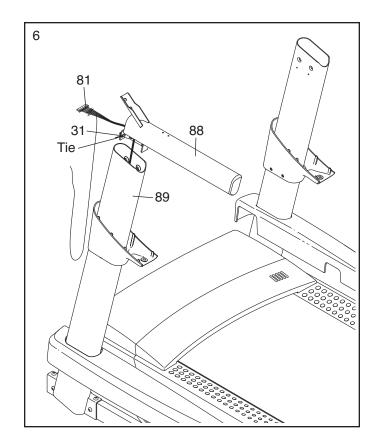
Attach the Left Handrail (88) to the Left Upright (89) with two 5/16" x 1" Bolts (5), two 5/16" Star Washers (11), and a 5/16" x 1 1/4" Bolt (4). Do not fully tighten the Bolts yet.
