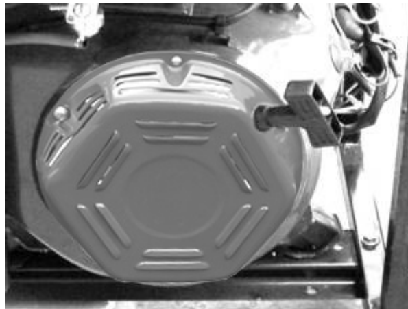
Figure 6 - Pull-cord for starting the engine.
