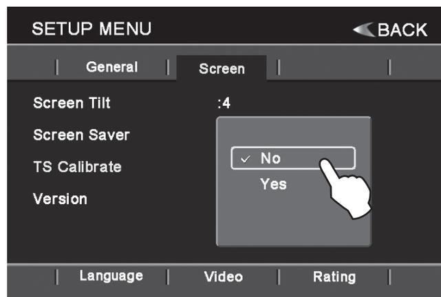
**Note:** For proper calibration you must touch each pointer for 2 seconds. If pointers are not touched properly, the calibration sequence will start over until the calibration is done correctly.
