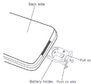
Remove the battery from the battery holder
