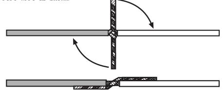
4. Use electrical tape to wrap, be sure to cover about 2 inches on either side of connection. Secure with wire ties as shown. Electrical Tape
