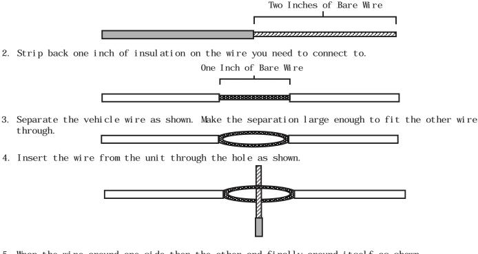
5. Wrap the wire around one side then the other and finally around itself as shown.
