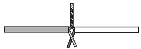
3. Lay upper twisted pair of wires over right wire as shown. Bring lower twisted pair of wires up to meet the left wire as shown.
