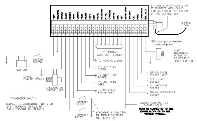
DIGITAL DASHBOARD WIRING DIAGRAM
