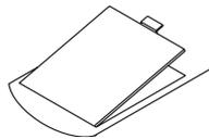
1. Press the battery compartment cover's tab and lift off the cover.
