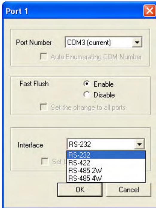
\* The UPort 1100 only supports RS-232. For this reason, when using the UPort 1100, the Interface drop-down box will be inactive.
