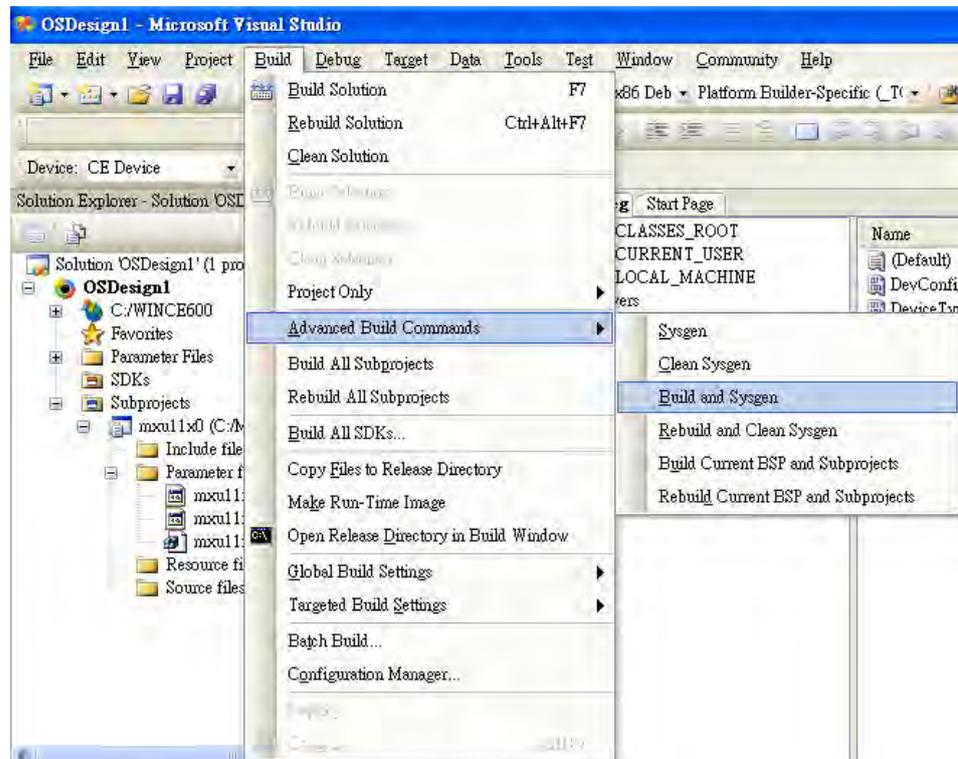
**Step 8:** After building sysgen, select **“Build”** and **“Make Run-Time Image”** to create the WinCE OS image. Finally, copy your image file to the target Host.
