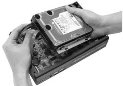
5. Secure the hard disk inside the unit then replace unit cover
