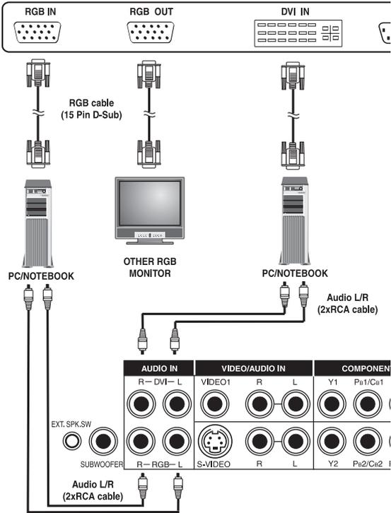
1. For most PC's, connect the 15-pin D-Sub **RGB** connector from the back of the PC to the **RGB-IN** connector located on the back of the display. If you have a PC that is equipped with a DVI (Digital Visual Interface), you may connect the PC DVI connector from the back of the PC to the DVI-In connector located on the back of the display.
