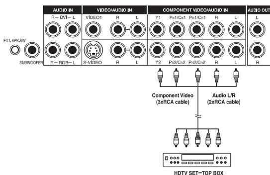
1. Connect the green (labeled as **Y**) jack from the HDTV Set-top box to the green **Y1** jack of the display.
