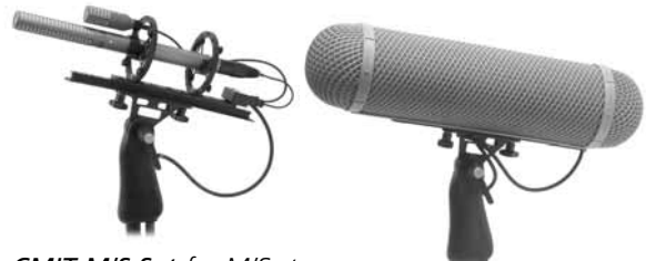
CMIT MIS Set for MIS stereo: CMIT 5 U shotgun microphone, WSR MS CMIT basket-type windscreen (100 mm dia., comprising elastic suspension with pistol grip and Connbox and a KMSC MIS double clamp), WJ CMIT Windjammer, CCM 8Lg figure-8 compact microphone
