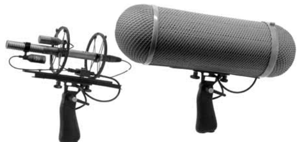
Double MIS Set "CMIT": CMIT 5 U shotgun microphone, elastic suspension with pistol grip and Connbox, WSR DMS CMIT LU basket-type windscreen (150 mm dia.), Windjammer WJ DMS CMIT, 2 × KMSC MIS double clamp, 1 × CCM 4Lg (cardioid), 1 × CCM 8Lg (figure-8)
