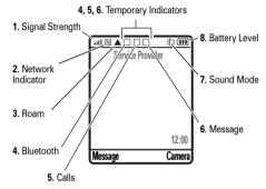
Signal Strength Indicator – Vertical bars show the strength of the network connection. Network services such as calls may not be available when \( \mathbb{T} \) or \( \mathbb{T} \) appears. 2 Network Indicator – Shows when your phone is using a GSM connection (standard network access), GPRS connection (high speed network access), 3G connection (highest speed network and video calling) or flight mode (no network connection, see page 74).
