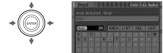
**4** The **Select City** screen is displayed. Use the joystick to enter a city name and scroll down to select that city. Press **ENTER** when finished.
