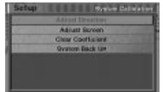
**3** The **direction correction** screen is displayed. Tilt the joystick toward the left and right to correct the direction.
