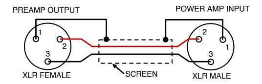
CONVENTIONAL: SCREEN CONNECTED AT BOTH ENDS
