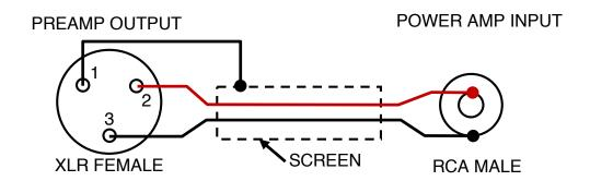
CABLE CONFIGURATION FOR XLR BALANCED PREAMP
