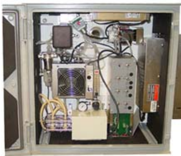
Figure 1-1. MicroCEM Sample Handling System
