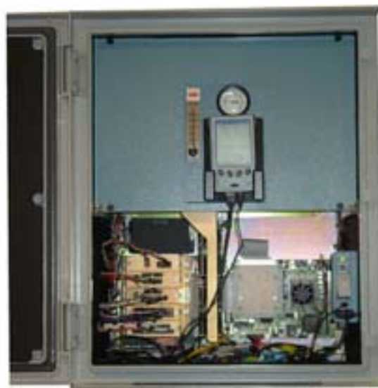
Figure 1-2. MicroCEM Continuous Emissions Monitor
