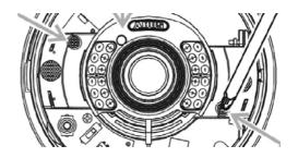
Place the base part to the desired installation position, mark the holes for fixing on the surface, and drill the fixing holes. Use the supplied screws and pegs to fix the base part on the surface. The cable rounting can be done to the side or throught the base.
