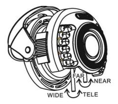
The fixing handles can be rotated anti-clockwise for defixing. Please perfom this with care to prevent the handles falling off the lens. Now please adjust zoom ratio and focus. Afterwards fix the handles by rotating clockwise.
