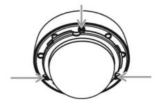
For this camera type the camera module can be removed, and it is fixed by two fixing screws. Base part of the camera and camera module are connected by a 15 pin D-Sub joint. Unscrew the fixing screws, and carefully remove the camera module.
