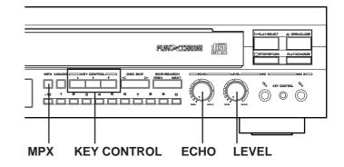
Adjusting the level of echo applied to sound signals input from the microphone(s)
