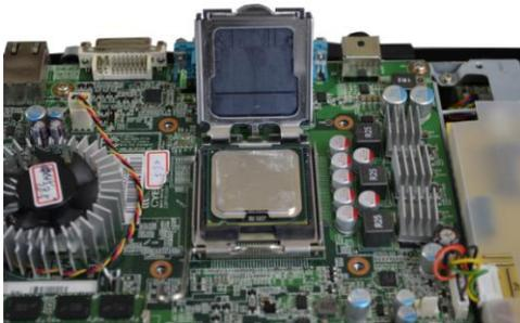
2. Raise the plastic cap to reveal the socket pins and open the cover by pushing down, pulling out and up on the lever beside the CPU socket.
