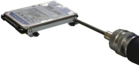
2. Slide the hard disk drive into the frame and line up the two screw holes accordingly. Secure the two screws on the Hard Disk Drive. Connect the SATA cable to the motherboard.
