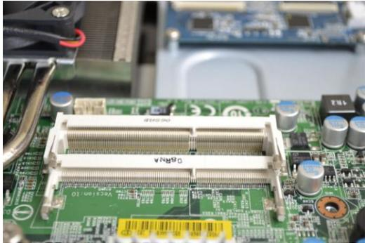
1. The memory module has only one notch and will only fit in the slot one way.
