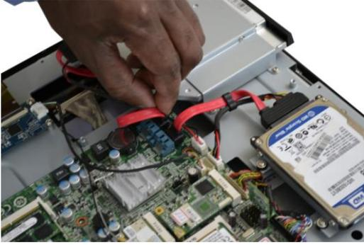
4. Connect the SATA cable. Connect the Power Cable.
