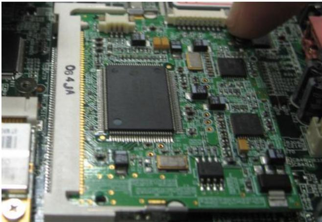
2. Press down the mini PCI card and the metal clip at each side of the mini PCI slot will automatically close.
