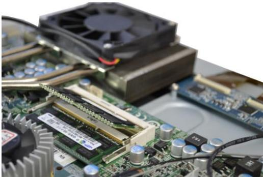
2. Insert the memory module into the DIMM slot at a 45° angle. Then push it in until the golden finger on the memory module is deeply inserted into the DIMM slot.
