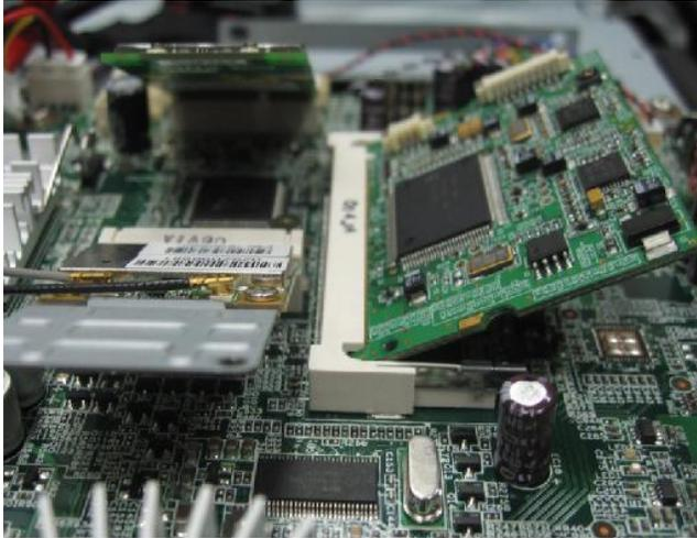
1. The mini PCI card has only one notch and will only fit in one way. Insert the mini PCI card into the mini PCI slot at a 45° angle. Then push it in until the golden finger on the mini PCI card is deeply inserted in the mini PCI slot.
