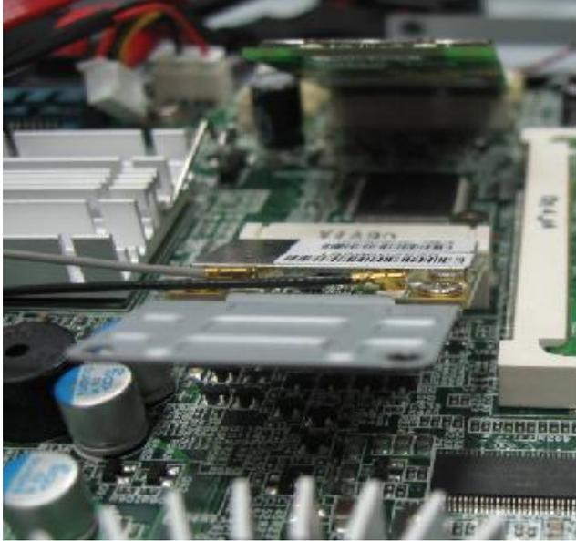
1. The mini PCIe card has only one notch and will only fit in one way. Insert the mini PCIe card into the mini PCIe slot at a 45° angle. Then push it in until the golden finger on the mini PCIe card is deeply inserted into the mini PCIe slot.
