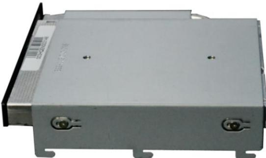
3. Secure the four screws on the ODD frame.
