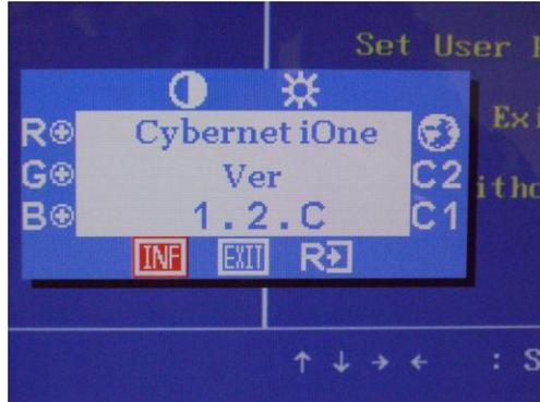
When the Menu button is pressed, the onscreen display appears as pictured above. When in Menu Mode you can move to the various icons with the – (left) or + (right) button. When you are at the icon you wish to adjust, press Menu again (Enter) to change the color of the icon and then toggle your desired adjustment by again pressing either – (left) or + (right). The screen will exit automatically in a matter of seconds if no selection is made.
