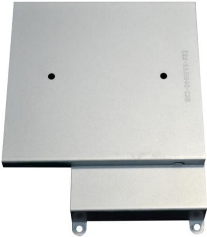
1. Remove back bezel as indicated in the iOne disassembly section. Remove the Optical Disk Drive frame.
