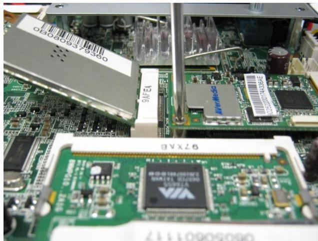
2. Press down the mini PCIe card and secure the screw to complete the installation.
