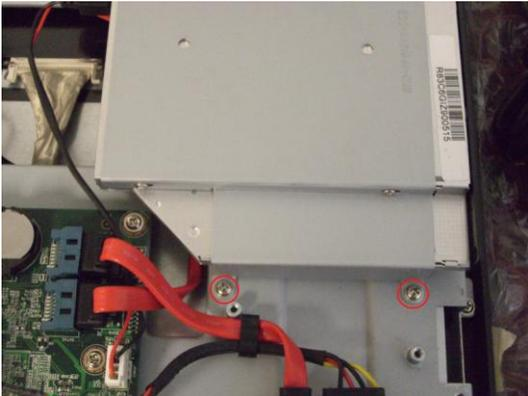
6. Install the ODD frame and line up the two screw holes over the Metal support.
