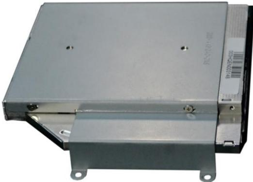
2. Put the ODD on the ODD frame and line up the four screw holes accordingly.
