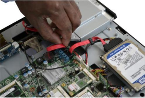
3. Connect the other end of the SATA/Power cable to the Hard Disk Drive as shown.
