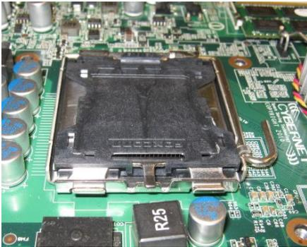
1. The socket has a plastic cap on it to protect the pins from damage. This should remain in place until actually installing a CPU.
