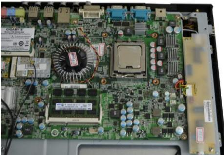
3. Install the CPU after confirming the direction for correct mating. Be sure to hold the CPU by the edge of the CPU base.
