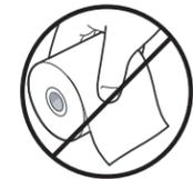
Paper must unroll from the bottom of the roll to insure that the image prints correctly.
