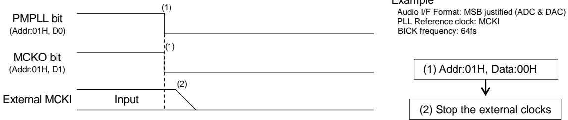
Figure 48. Clock Stopping Sequence (3)
