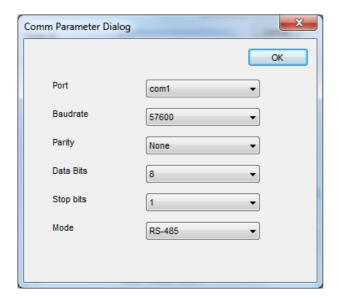
For HMIs with a single 9 way d-type connector select "Com1" as the required port. If the HMI has more than one serial port set 'Port' to match whichever port is physically wired.
