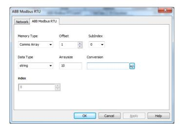
The 'ArraySize' field in the dialog determines the number of characters the string Tag can store. In this case 10 characters means the HMI will access COMMSINTEGER(1), COMMSINTEGER(2) and the top 16 bits of COMMSINTEGER(3).
