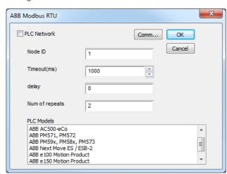
If the HMI is connected to a single Modbus RTU slave device (e.g. e100 controller or AC500 PLC) there is no need to select the 'PLC Network' check box. If there are multiple slave devices connected to the HMI then it is essential this box is selected (for the purposes of this application note we will select this option).
