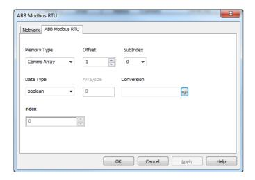
The field tab lets us program which memory location in the motion controller the Tag relates to. The available 'Memory Type' selections are specific to the PLC model selected as shown by the table below:
