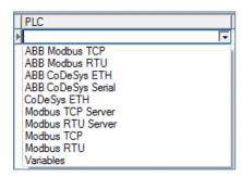
We need to select the ABB Modbus RTU protocol. This is a client (master) protocol that allows the CP600 HMI to communicate with both ABB PLCs and motion control products. The ABB versions of Modbus protocols differ from the generic Modbus protocols available in two ways:
