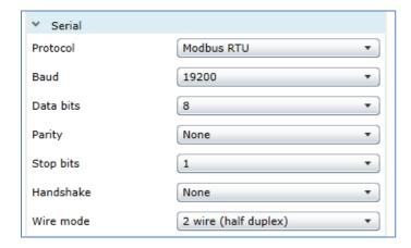
The other settings on this dialog should be made to suit the connection to the HMI (this is detailed later when discussing the protocol setup in the HMI project).
