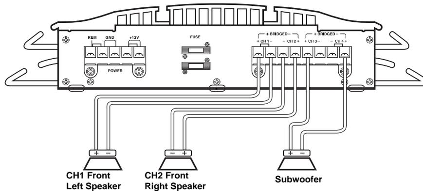
**Note:** **CH4 (+)** is used as a negative (-) terminal for a bridged connection.
