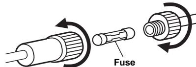
3. If the fuse is blown, replace it. Use only an SFE-type fuse with the proper rating (available at many automotive supply stores). The fuse must be 60 amps.
