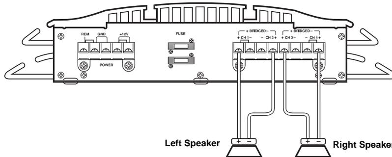
**Caution:** This connection produces 200 watts per channel. Use this connection only if you have high-power speakers that can handle a power output of 200 watts.
