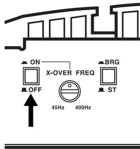
**Note:** X-OVER FREQ selects the limit at which the amplifier will pass frequencies (from 45–400 Hz). You should not use it to adjust the sound you hear through your main speakers.
