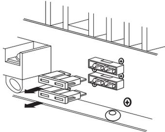
3. If the fuse is blown, replace it. Use only a blade-type fuse with the proper rating. The fuse must be 30 amps.
