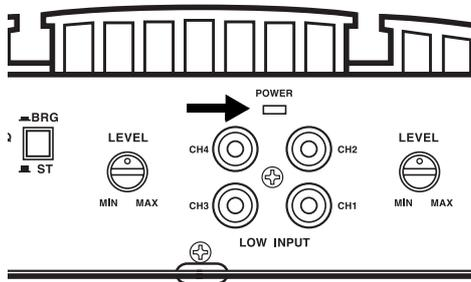
**Important:** Your amplifier requires 60 amps or more of power from your vehicle's battery during operation. To protect your battery from discharging, do not operate the amplifier unless your vehicle is running.
