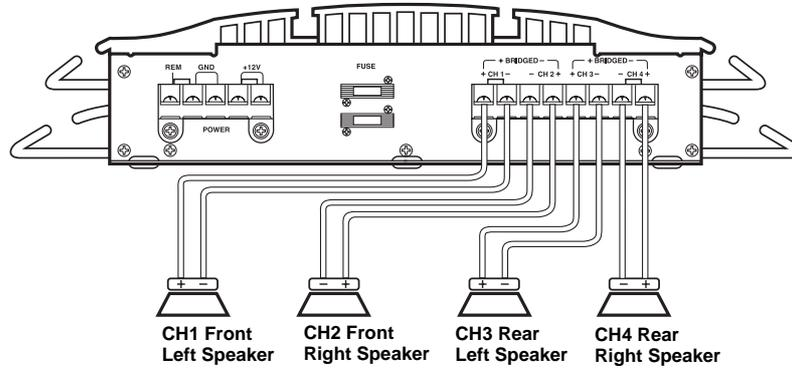
1. Use a screwdriver to connect the front left speaker's positive (+) wire to the amplifier's **CH1 (+)** terminal.
