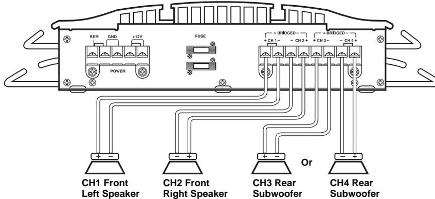
1. Use a screwdriver to connect the front left speaker's positive (+) wire to the amplifier's CH1 (+) terminal.
