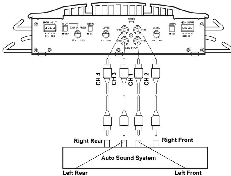
*If your auto sound system has two line out jacks (left and right), connect the auto sound system to the amplifier.*
