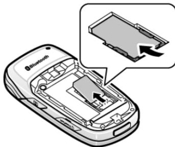
6. Place the battery so that the 3 brass tabs on the end align with the 3 brass prongs at the bottom of the battery compartment (1). The arrow on the battery should be pointing down. Press the battery down until it clicks into place (2).
