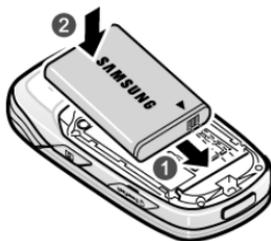
7. Replace the battery cover. Make sure that the battery is properly installed before switching on the phone.
