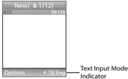
1. To change the text input mode, press the Right soft key.
