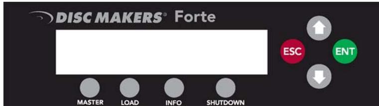
Figure 1-4 LCD Control Panel Layout
