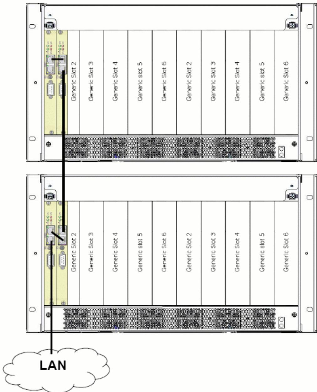
Figure 15: Connecting two MS430502M chassis with 2nd ethernet port
