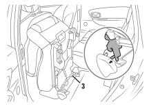
Lift it as far forward as possible (2) until control **3** locks (move the front seat forward if necessary), lower it until it is 10 centimetres from the floor and release it. Check that it is correctly locked. Refer to the label located on the back of the seat.
