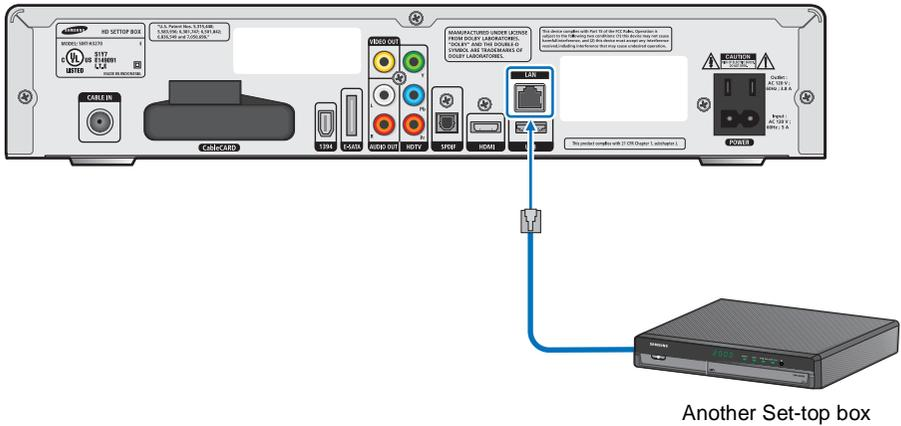
Connect the **LAN** port on the rear of the STB with the **LAN** port of another STB by using an Ethernet cable.
