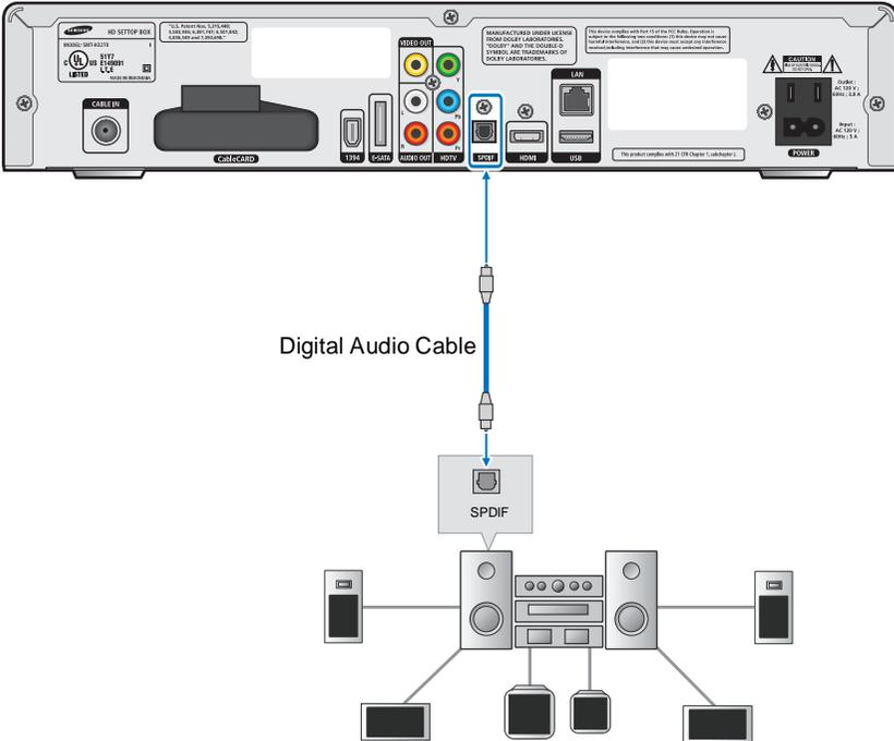
Using an Optical cable, connect the **SPDIF** port of the Dolby digital amplifier to the **SPDIF** port on rear panel of the STB.
