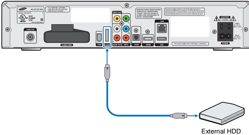
Connect the **E-SATA** port on rear of the STB with **E-SATA** port of external HDD by using E-SATA cable.
