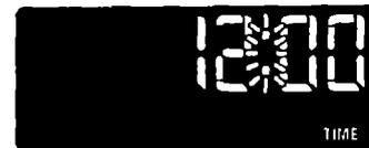
2. Use the Hour and Minute pads to set the time of day. Push the "up" (▲) or "down" (▼) pad(s) until the correct time shows in the display.
