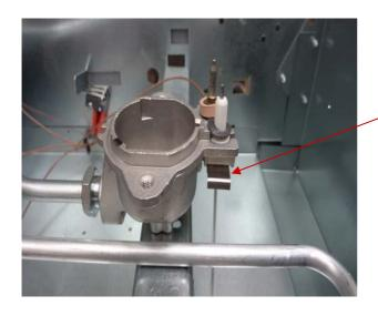
FOLLOW STEP 2 AND 3 AND REMOVE THE HOTPLATE AND FACIA PANEL REMOVE ELCTRODE CLIP BY SQEEZING TOGETHER AND PULLING TO REMOVE REMOVE ELECTRODE FROM BURNER BOWL AND IGNITION LEAD FROM IGNITION GENERATOR ON REPLACING ALWAYS ENSURE THAT THE RUBBER WASHER IS REFITTED
