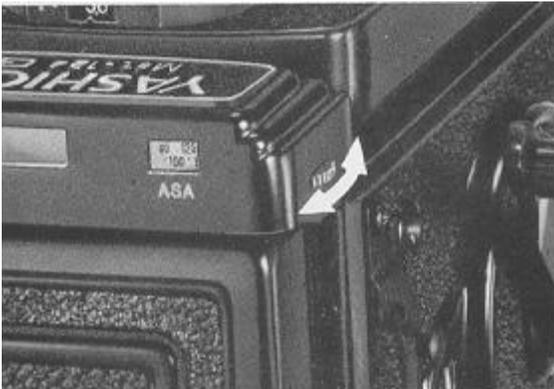
1. Turn the ASA Film Speed Setting Wheel until the figure denoting the ASA rating of the film in use aligns with the red indicator in the ASA Film Speed Indicator Window...
