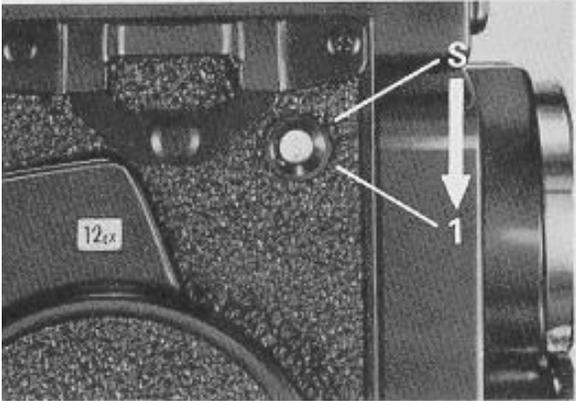
9. The letter "S" appears in the Exposure Counter during the film loading operation. After closing the Back Cover, wind the crank-handle until the figure "1" appears in the Exposure Counter Window.
