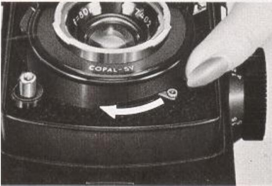
When using the self-timer, always see to it that the Flash Synchronizer Selector is switched to "X" position
