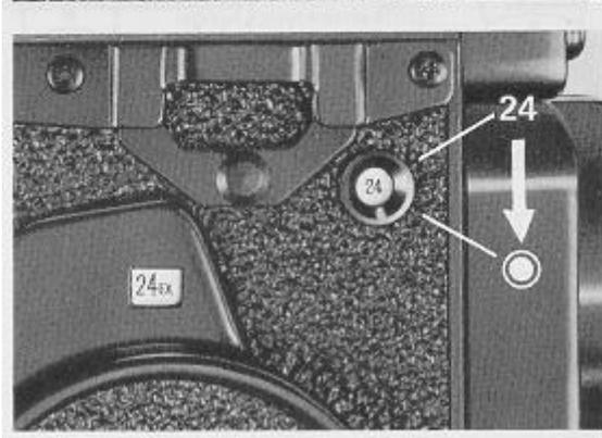
1b. When the figure "24" appears in the exposure counter window, it signifies that the full length of the film has been exposed. Another wind of the crank-handle will bring out the Mark in the window, but continue winding until the crankhandle turns freely without tension.
