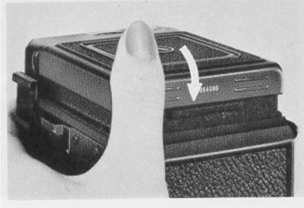
2. When the camera is to be left unused, fold the focusing hood. This will switch off the meter and prevent draining of battery power.
