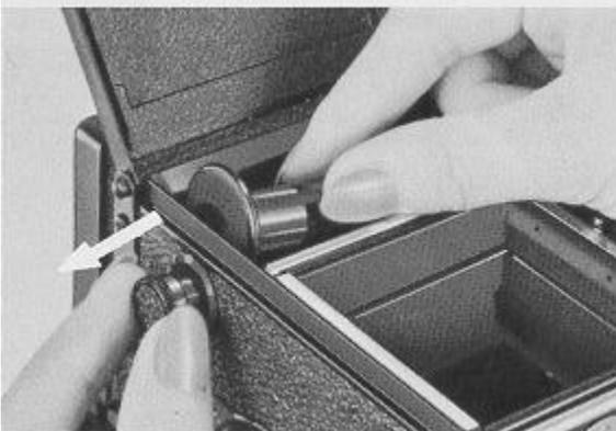
2. Pull out the Upper Spool Holder **Knob** and place the empty spool in the Take-Up Spool Chamber. After the Take-up Spool is set properly in the camera, return the **Spool Holder Knob** to its original position.
