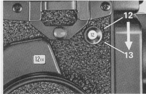
1. When the figure "12" appears in the exposure counter window, it signifies that the full length of the film has been exposed. Another wind of the crank handle will set the exposure counter between "12" and "13", but continue winding until the crank-handle turns freely without tension....
