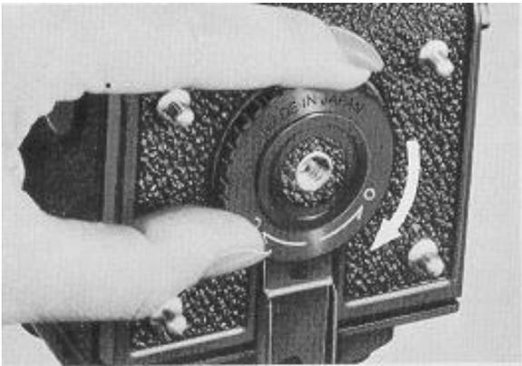
8. Then, close the Back Cover and turn the Back Cover Locking Ring toward "C" (Close) while pressing the cover. (When closing the Back Cover, see that the lug on the body rests properly in the slot on the Back Cover Latch.)
