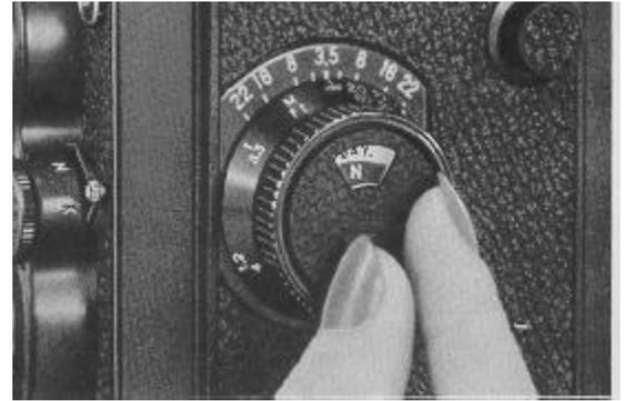
After loaded the film, turn the Film Type Indicator as illustrated, so that the letters equivalent to the film type in use are indicated in the window.
