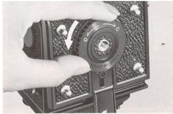
3. Pull out the Upper Spool Holder Knob and take out the exposed film from the film chamber. Paste the seal to prevent recoiling and wrap the film in light-proof paper.
