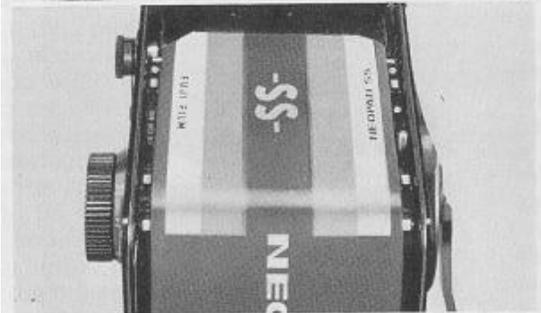
[5] Draw out the film leader gently and introduce its tip straight and amply into the slot on the spindle of the Take-up Spool. The film may fail to advance if the film leader is not inserted properly into the slot.
