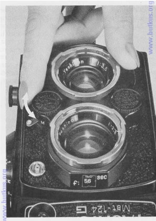
Turn the Aperture Control Dial and coincide the yellow follower needle (coupled to the aperture mechanism) with the red meter pointer (coupled to the shutter mechanism), both visible in the Exposure Indicator Window.
