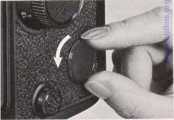
1. Open the Battery Compartment Cover holding with finger and by turning it counter-clockwise. This camera uses a 1.3 V mercury battery to power its exposure meter. Use either Mallory PX-13B, Eveready EPX-13 or equivalent.
