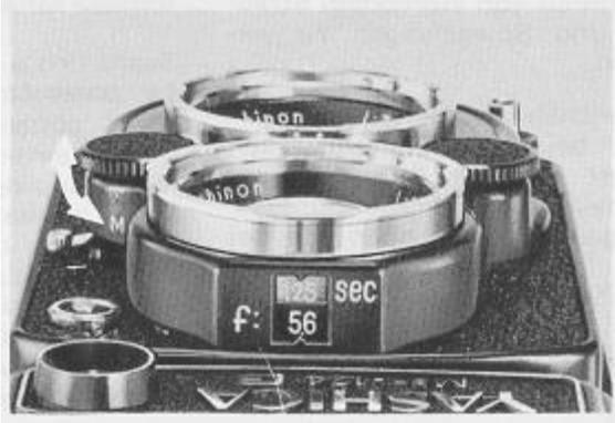
In case the correct combination of shutter speed and aperture is 1/250 sec. and F8, turn the Aperture Control Dial and set the lens aperture to F5.6 when using a Y2 filter.
