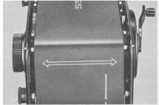
7b. Continue winding the film until the "start" mark on the film leader paper lines up with the RED triangular (▶) "start" mark for 220 film....
