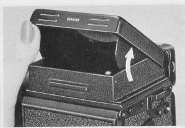
1. The exposure meter begins to function when the focusing hood is set upright by lifting it W gently with your fingertip...
