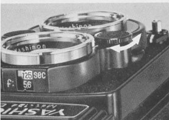
2. Center the desired shutter speed in the Shutter Speed Indicator Window by turning the Shutter Speed Control Dial. The exposure meter pointer in the Exposure Indicator Window is coupled to the shutter mechanism and will shift in either direction when the shutter speed is adjusted.
