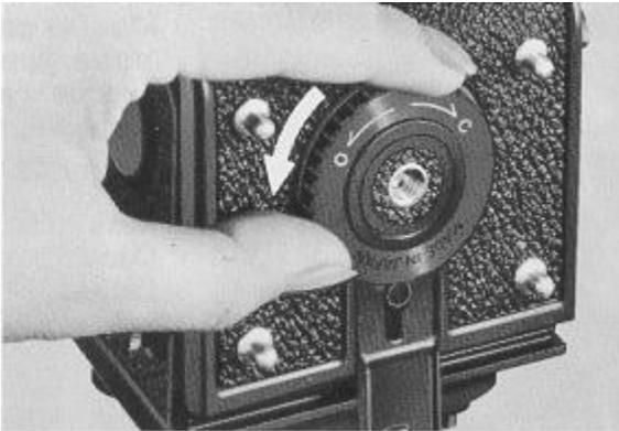
1. The Back Cover will spring open when the Back Cover Locking Ring is turned in the direction of "O" (Open).
