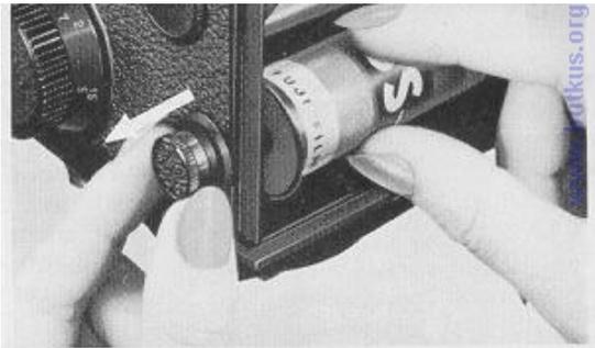
[4] Place the new roll of film in the lower film chamber while pulling out the Lower Spool Holder Knob. Also make sure that the Lower Spool Holder is returned to its original position after loading the film.
