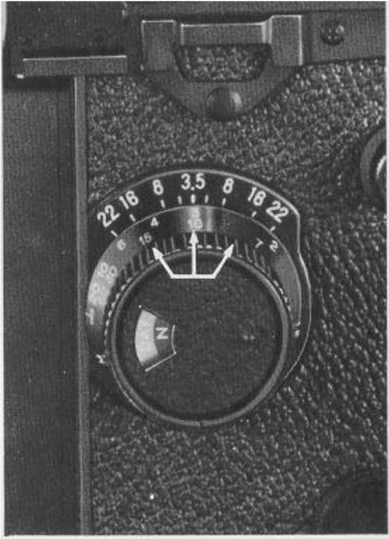
The depth of field for a given aperture and camera-to-subject distance can be read off the depth-of-field scale around the Focusing Knob. By checking this scale, you can easily determine before shooting the extent over which the objects will appear sharp and clear.---
