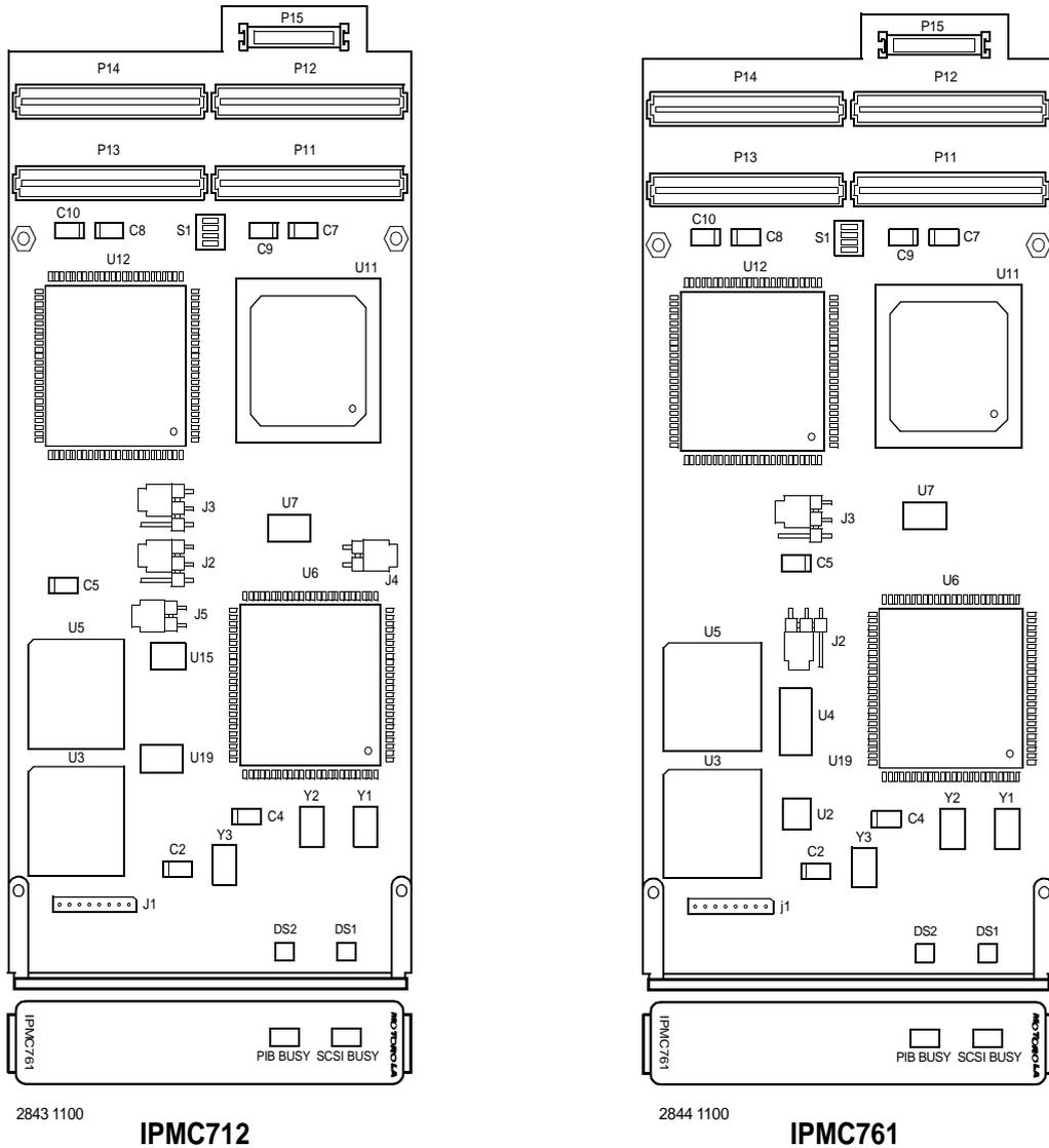
**Figure 1-1. IPMC Component Layout**
