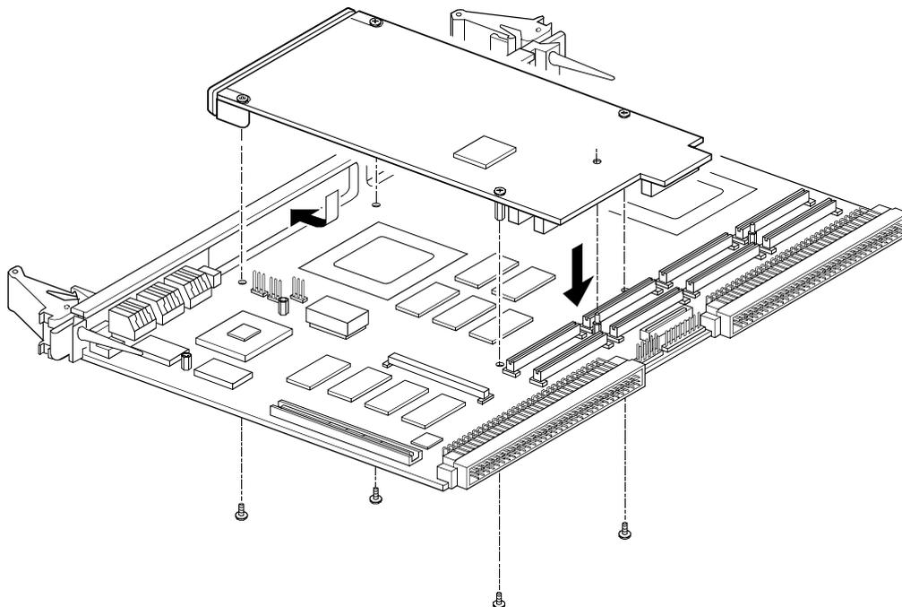
**Figure 2-1. IPMC Installation**
