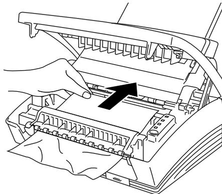
Fig. 6-6 Paper Jam Inside the Printer
