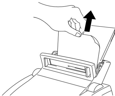
**Fig. 6-4 Paper Jam in the Feeder**
