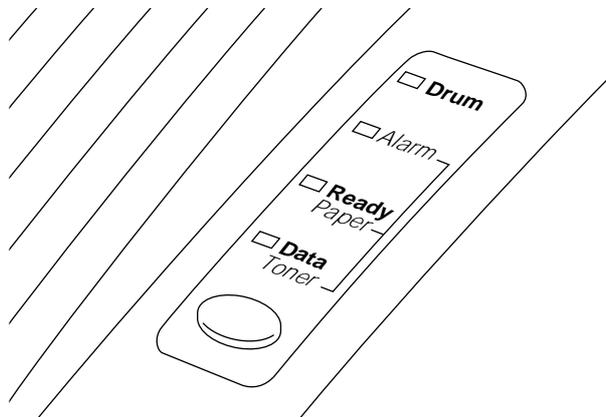
Fig. 3-1 Lamps and Switch on Control Panel
