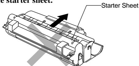
Fig. 5-14 Do Not Remove the Starter Sheet
