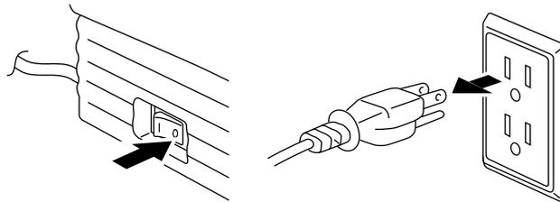
Fig. 5-19 Turning off the Switch and Unplugging
