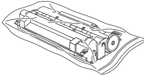
**Fig. 5-25 Placing the Drum Unit in the Plastic Bag**
