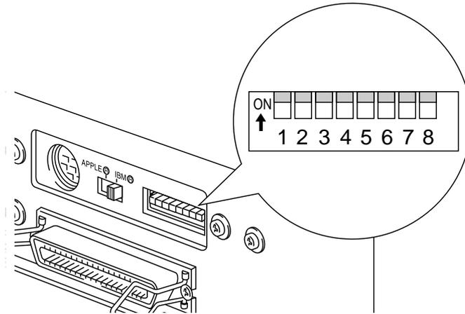
**Fig. 4-2 Setting the Serial Interface Parameters**
