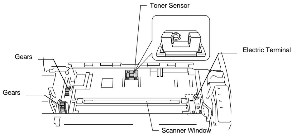
**Fig. 5-22 Cleaning the Gears, Electric Terminals, Scanner Window, and Toner Sensor**
