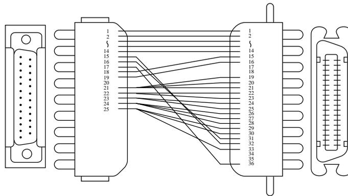
Fig. A-1 Parallel Interface Cable
