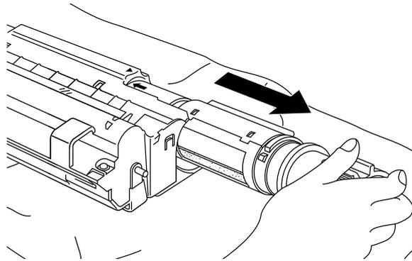
Fig. 5-12 Removing the Toner Cartridge
