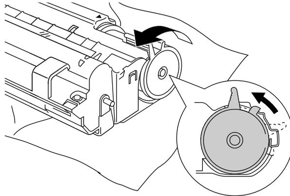
Fig. 5-4 Turning the Lever to Close the Shutter
