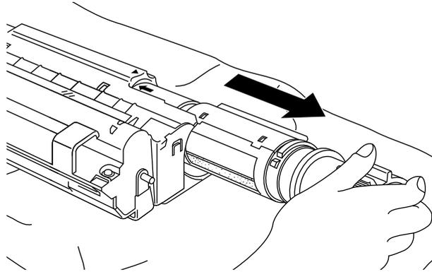
Fig. 5-5 Removing the Old Toner Cartridge
