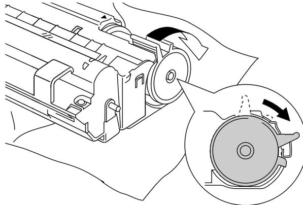
**Fig. 5-8 Turning the Lever to Open the Shutter**
