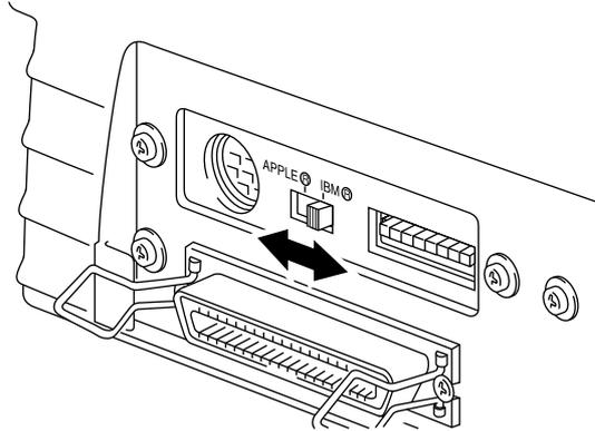
Fig. 4-1 Selecting the RS-422A (Apple) or RS-232C (IBM) Serial Interface
