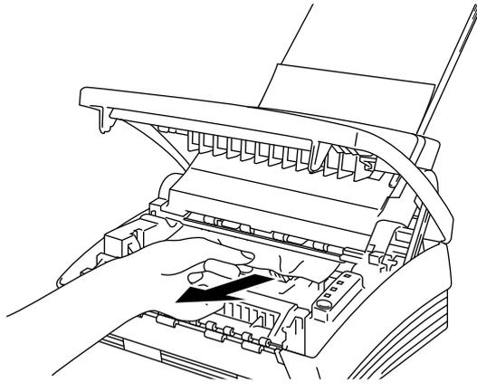
Fig. 6-5 Paper Jam near the Drum Unit
