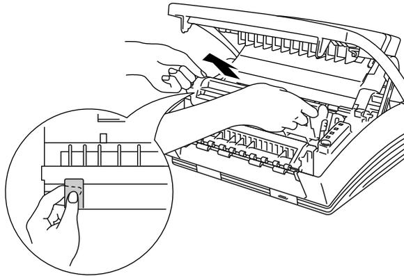
Fig. 5-24 Removing the Drum Unit Assembly
