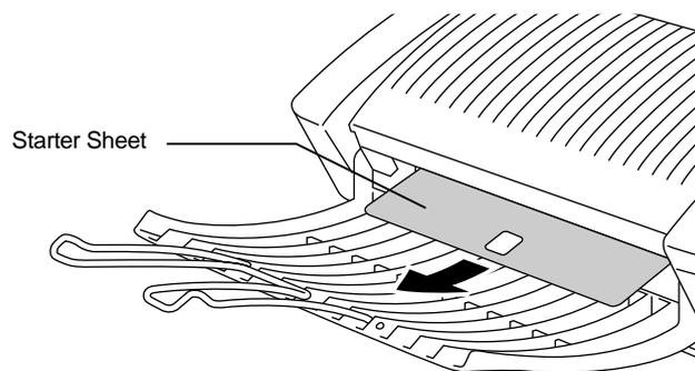
**Fig. 5-16 Ejecting the Starter Sheet**
