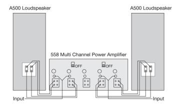
Extremely high sound quality can be achieved using two separate channels of the multi channel power amplifier to drive the LF and HF units in each loudspeaker.
