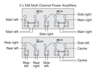
Two 558 Multi Channel Power Amplifiers can be used as the basis of a superb seven-channel surround system, taking advantage of bridged mode operation to give more than twice the power output for the three front channels.
