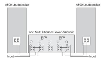
You can wire channels 1/2 and 4/5 in bridged output mode, to obtain more than twice the power output.
