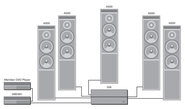
The 558 Multi Channel Power Amplifier is ideal for use with the Meridian 561 Digital Surround Controller or the 568 Digital Surround Processor, to drive five analogue loudspeakers in a high-quality surround system. The 568 provides balanced
