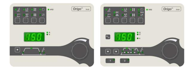
Welding process parameters are controlled via the control panel. See the separate instruction manual for a detailed description of the panels.
