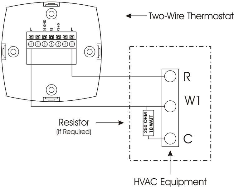
If the Two-Wire thermostat is losing time or showing PF or P- it may be necessary to install the 10 watt 250 ohm resistor that is supplied with the thermostat.
