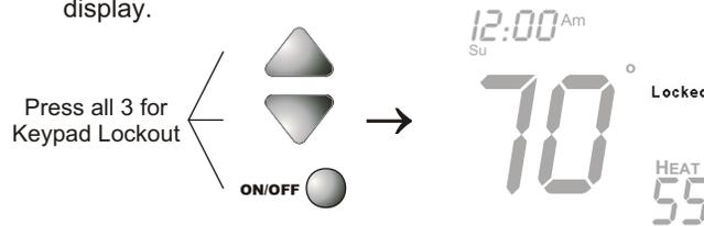
To **unlock** the buttons, again press and hold the On/Off button. While holding the On/Off button in, press the Up and Down buttons in together. The **Locked** icon will disappear from the display.
