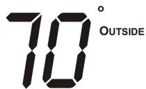
Pressing the Outside button will display the outside temperature. A subsequent press of the Outside button will return the display to the previous screen. Normal operation will continue while the Outside temperature is being displayed.
