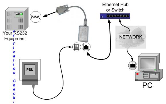
If powered up correctly, the NetPort power LED will light yellow and remains on. This LED is on the RS232 end.
