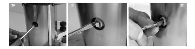
The task of the carbon brushes is to transport the power to the armature via the rotating collector. There are two carbon brushes. They should be checked regularly and changed in pairs after approx. 100 hours normal operating time.
