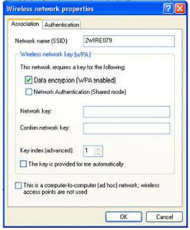
• Enter the 10-digit encryption key from the bottom of the Gateway into the **Network key:** field and again in the **Confirm network key:** field. Click the **OK** button.
