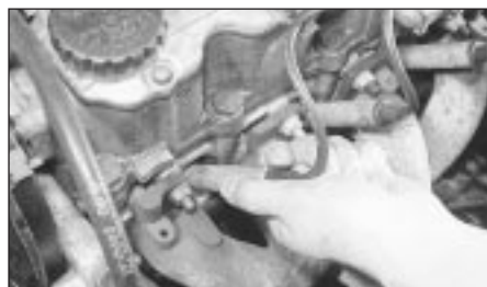
A Check that the spark plug HT leads are securely connected by pushing them home.
