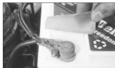
D Check the security and condition of the battery connections.
