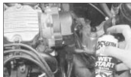
E Check that the ignition coil wiring plug is secure, and spray with water-dispersant if necessary.
