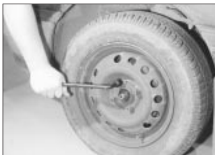
4 Remove the wheel trim (where fitted) and slacken each wheel bolt by half a turn.
