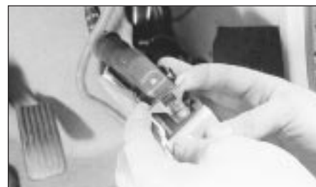
C Check the ECU multi-plug for security (where fitted), with the ignition switched off.
