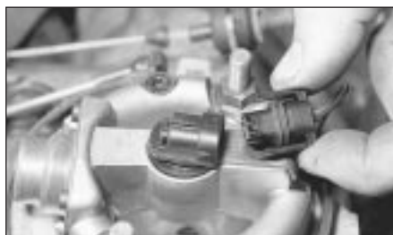
B The fuel injection system wiring plug may cause problems if not connected securely.
