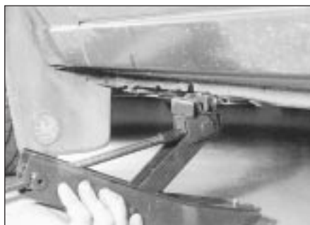
5 Raise the jack whilst locating below the jacking point (ensure that the jack is on firm ground and located correctly)
