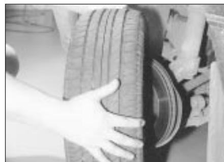
6 Turn the handle clockwise until the wheel is raised clear of the ground. Remove the bolts and lift the wheel clear.
