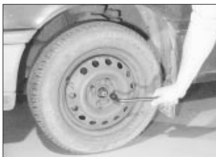
7 Position the spare wheel and fit the bolts. Hand tighten with the wheel brace and lower the car to the ground. Tighten the wheel bolts in a diagonal sequence.
