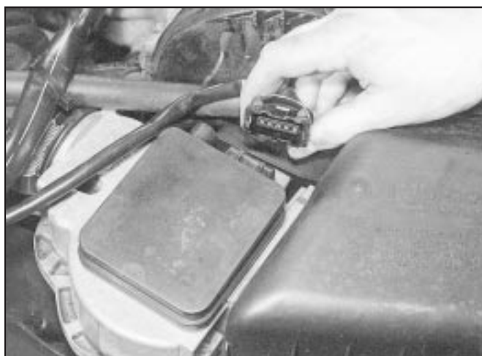
Check that electrical connections are secure (with the ignition switched off) and spray them with a water dispersant spray like WD40 if you suspect a problem due to damp
