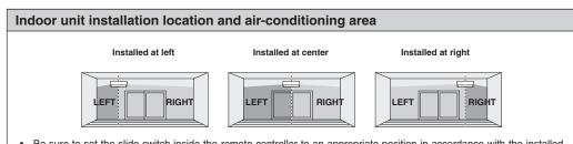
· Be sure to set the slide switch inside the remote controller to an appropriate position in accordance with the installed position of the indoor unit. If the switch is not set correctly, the air conditioner may not function properly. (Refer to page 4.)
