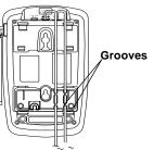
6. Align the keyhole slots with the mounting screws and slide the base downward to secure it.
