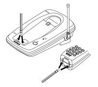
If the battery pack becomes completely discharged or the base loses power while the handset is away, the security access-protection code needs to be reset. To reset the code, return the handset to the base for about 5 seconds. If it was the handset that lost power, leave the handset on the base to recharge the battery pack
