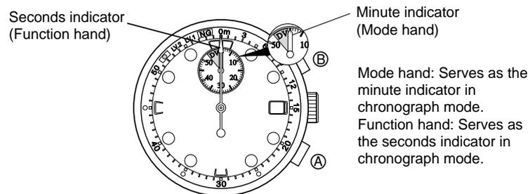
\* If the watch is left in reset status in the chronograph mode for 3 minutes, it automatically switches to the Time mode.
