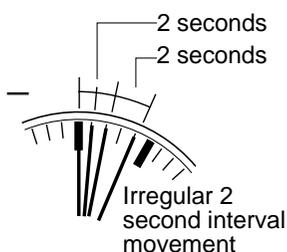
To change the watch to the time mode, reset the watch correctly after sufficiently charging the battery.
