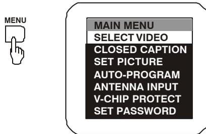
2. Press the CHANNEL ? or ? buttons to highlight the function.
