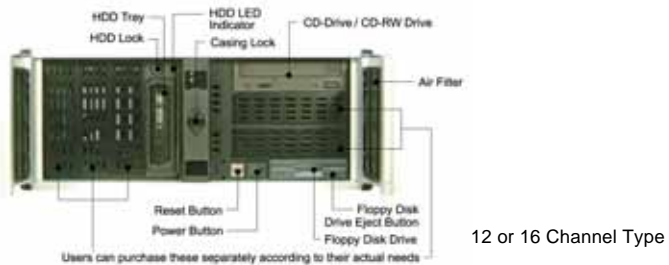
Figure 1-2: Front Inside View of the Digital Video Recorder
