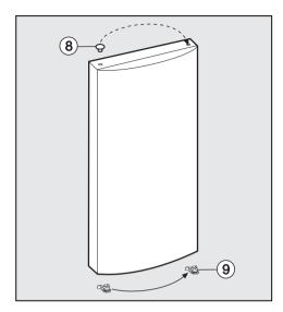
Remove cap (a) from the bearing bush in the door and refit on the opposite side.
