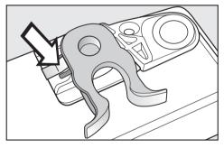
Remove clamp (9) from underneath the door and fit it on the opposite side.
