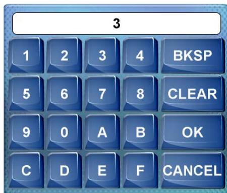
Touch **CLEAR** to remove any previous entry. Then enter the ID required. Touch **OK** to accept the entry or **CANCEL** to cancel the entry. This hides the hex keypad and returns the display to the “**Edit IP Table Entry**” screen.
