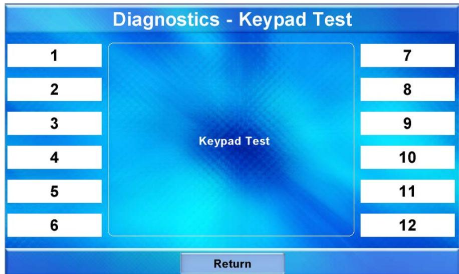
The **Diagnostics – Keypad Test** screen allows testing of the hard keys on the touch screen faceplate (assuming the button faceplate and not the no-button faceplate is installed). Pressing any of the hard keys results in its corresponding section of the screen changing (from a black number on a white background to a white number on a dark background) in recognition of the key press. Touch **Return** to go back to the **Diagnostics** menu.
