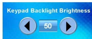
Use the **Keypad Backlight Brightness** controls to adjust the relative level (0% to 100%) of current key backlighting. Use the **Key Brightness Level – HIGH** and **Key**
