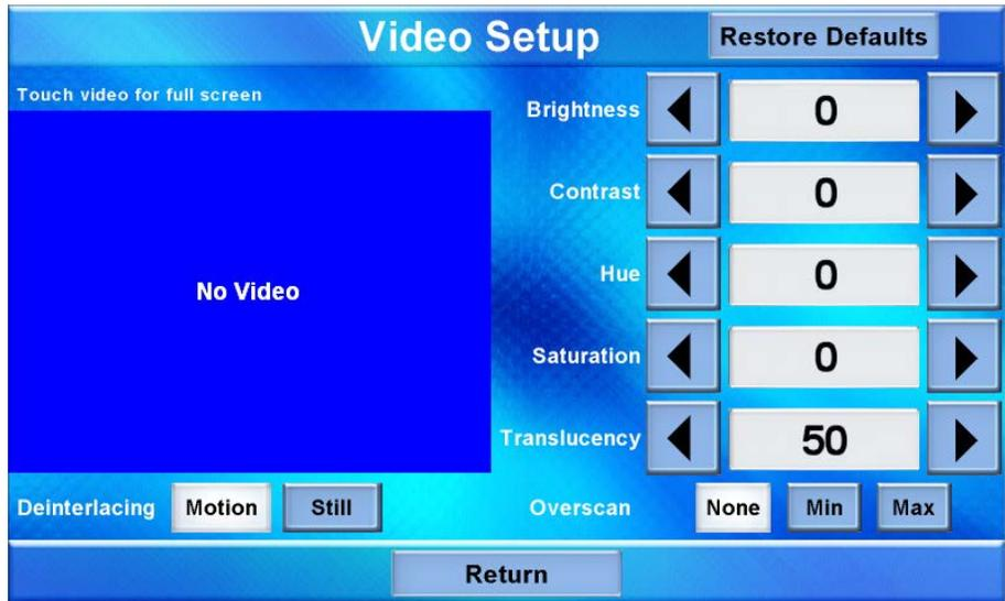
The **Video Setup** screen contains buttons for adjustment of **Brightness**, **Contrast**, **Hue**, **Saturation**, **Translucency**, type of **Deinterlacing** and amount of **Overscan**.
