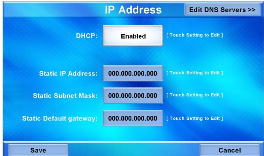
DHCP is enabled by default. To enter a **Static IP Address**, **Static Subnet Mask** or **Static Default gateway**, first touch the **DHCP Enabled** button. The button text changes to **Disabled**. Then touch the appropriate button for the address to be entered (or changed). A numeric keypad opens, as shown in the illustration that follows.
