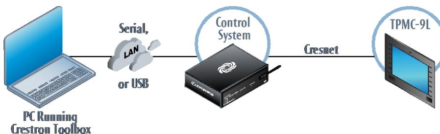
TPMC-9L connects to control system via Cresnet:
