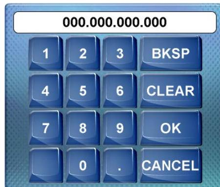
Touch **CLEAR** to remove any previous entry. Then enter the address required. Touch **OK** to accept the entry or **CANCEL** to cancel the entry. This hides the numeric keypad and returns the display to the **IP Address** screen.
