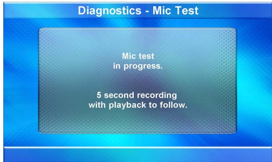
This screen performs a test of the TPMC-9L's built-in microphone. The touch screen records audio for five seconds and then plays back the recorded sound. Speak into the microphone on the front of the TPMC-9L and the recording is played back to confirm the microphone is functioning. When playback is finished, the display goes back to the **Diagnostics** menu.
