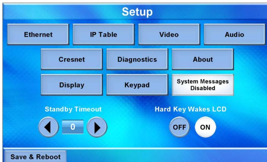
The **Setup** menu provides access to all basic functions and parameters. There are buttons for **Ethernet**, **IP Table**, **Video**, **Audio**, **Cresnet**, **Diagnostics**, **About**, **Display** and **Keypad**. There are also buttons to increase and decrease **Standby Timeout**, buttons to turn the **Hard Key Wakes LCD** function on or off, as well as a button to enable/disable system messages. A **Save & Reboot** button is provided to save settings and reboot the touch screen.
