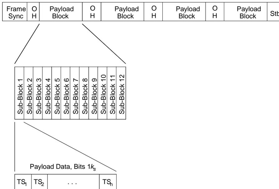
**Figure 11. G.shdsl frame order diagram with CAS signaling**
