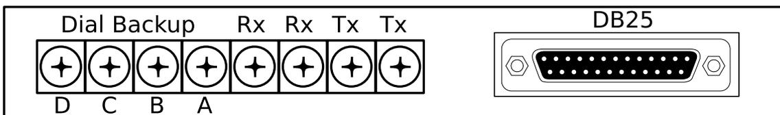
Figure 5. DM991S/SE Back Panel
