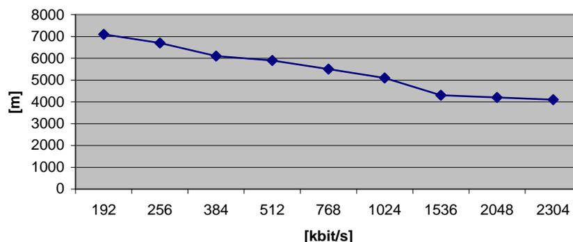
Figure 13. G.shdsl Interface Reach (m X kbit/s)
