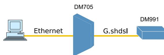
Figure 14. DM991 Managed as DM705 remote
