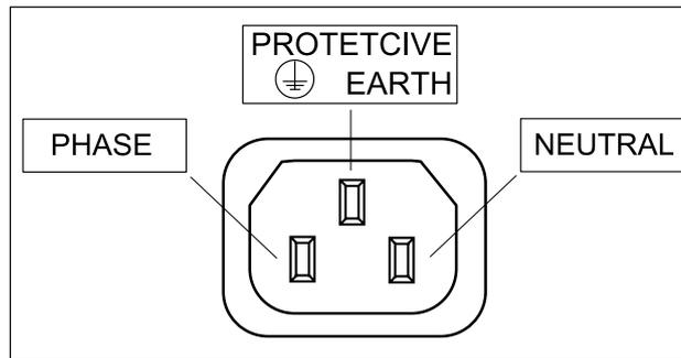
**Figure 38. Power Cable Pinout - DM991C/CE**
