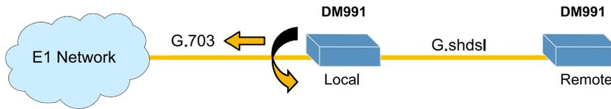
**Figure 28. DM991 - LAL Test on E1 Interface**
