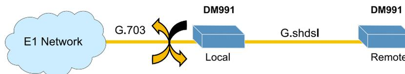
**Figure 27. DM991 - LDL Test on E1 Interface**
