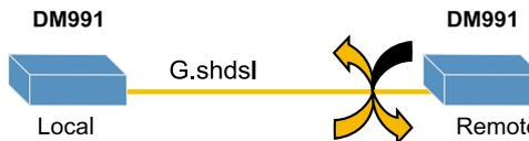
**Figure 26. DM991 - RDL Test on G.shdsl interface**
