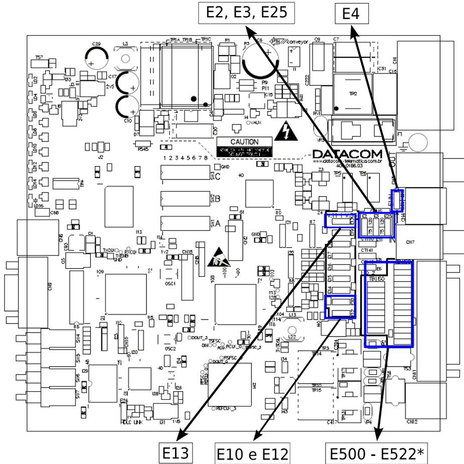
Figure 36. DM991C/CE – Map of Straps (PCI rev. 03 ou inferior)
