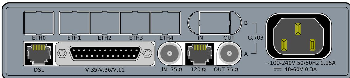
**Figure 10. DM991C/CE Back Panel**
