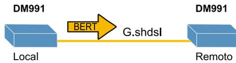
**Figure 25. DM991 - BERT Test on G.shdsl Interface**
