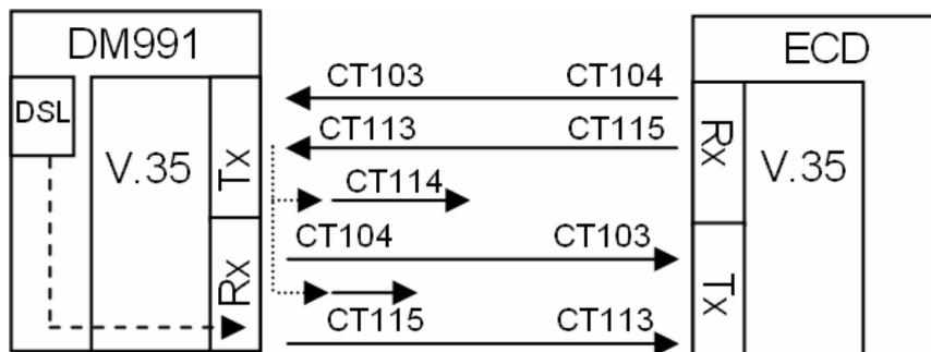
Figure 20. Digital Interface Operation with CT104 sinc. CT113
