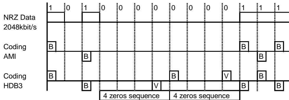
Figure 34. HDB3 coding in the G.703 2048kbit/s Interface
