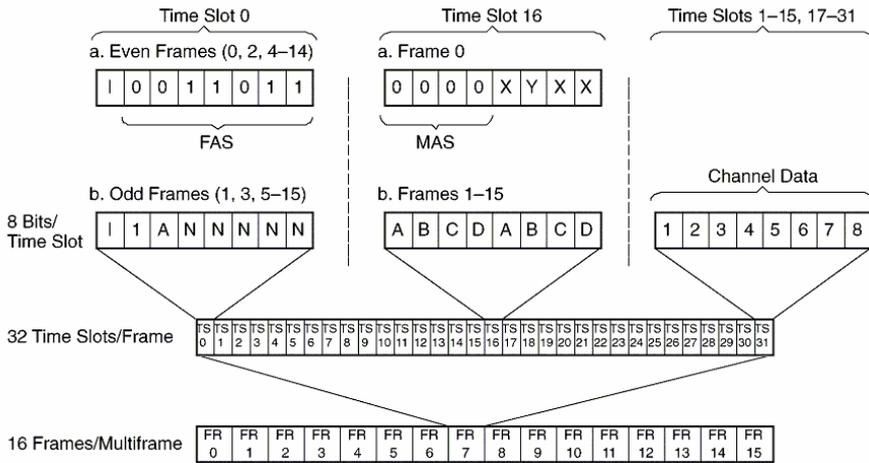
**Figure 33. ITU-T G.707 E1 frame structure recommendation**
