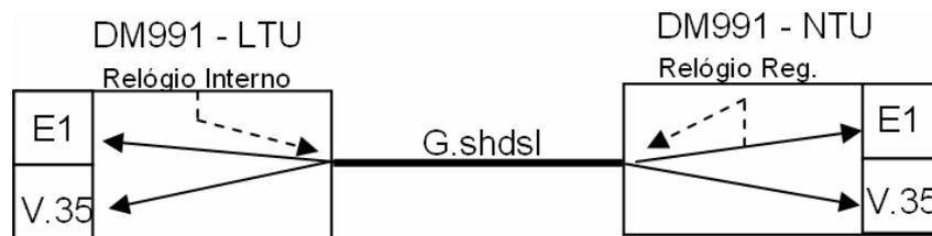
**Figure 15. Internal and Regenerated Clocks in Plesiochronous Mode**
