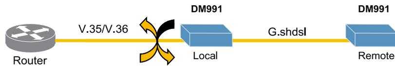
**Figure 29. DM991 – LDL on Digital interface**
