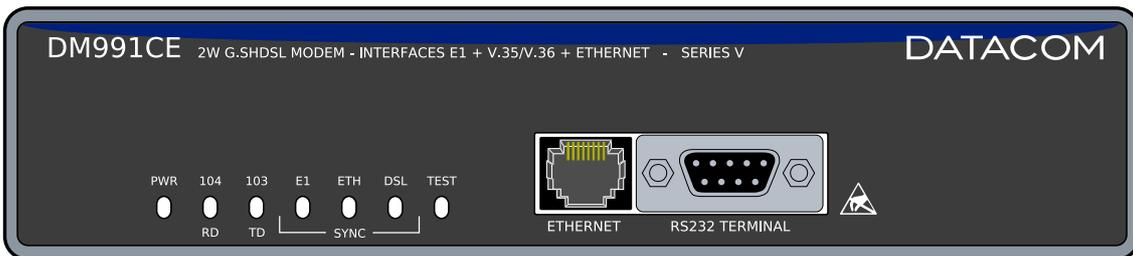
Figure 7. DM991CE 2W Front Panel
