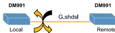
Figure 23. DM991 - Local Digital Loopback on G.shdsl Interface
