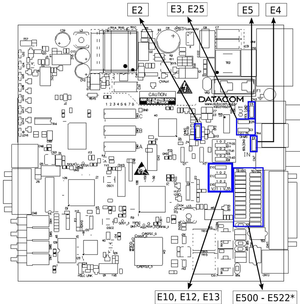
Figure 37. DM991C/CE – Map of Straps (PCI rev. 03 ou superior)
