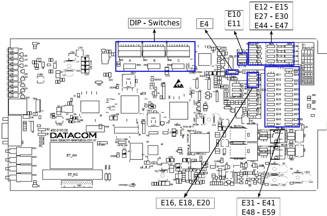
Figure 35. DM991S/SE - Straps and DIPs map
