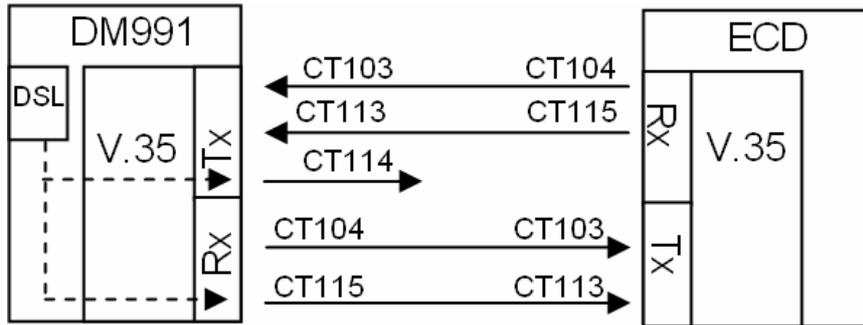
Figure 21. Digital Interface with CT113 Unlooped to CT114
