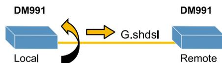
Figure 24. DM991 - Local Analogue Loopback Test on G.shdsl Interface
